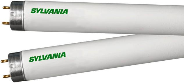
SYLVANIA OCTRON 800 XP XL ECOLOGIC3 lamps feature eXtended Life benefits of up to 75,000 hours life on instant start ballasts and 84,000 hours life on programmed rapid start ballasts. The life ratings reflect up to 88% longer life than T8 XP or XV lamps, which is the equivalent of an additional 8 years of maintenance-free lighting for typical operating cycles of 4,000 hours per year.
