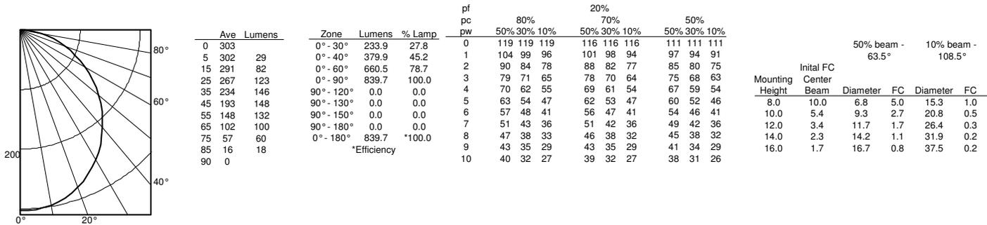
**WF4 LED 30K40K50K, 5000 K LEDs, input watts: 10, delivered lumens: 791, LM/W=79, test no. ISF 36826P6**
