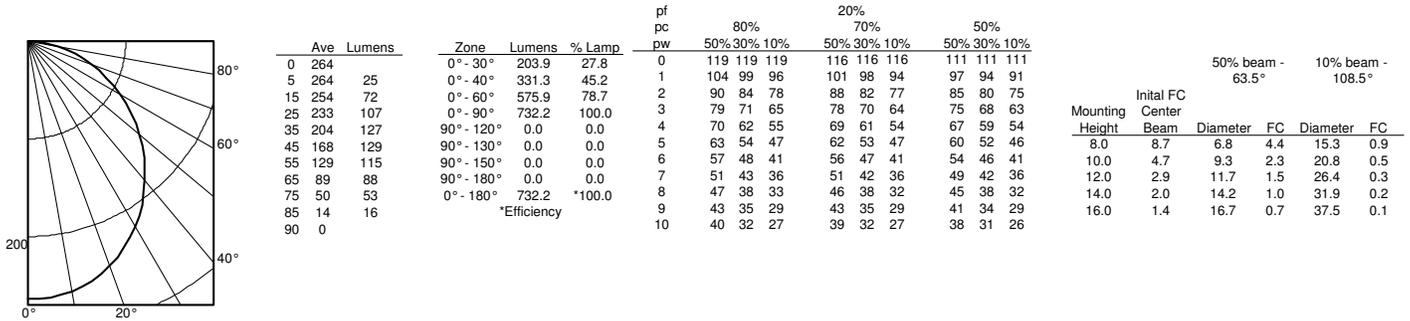
**WF4 LED 27K30K35K, 3000 K LEDs, input watts: 10, delivered lumens: 830, LM/W=83, test no. ISF 36826P2**
