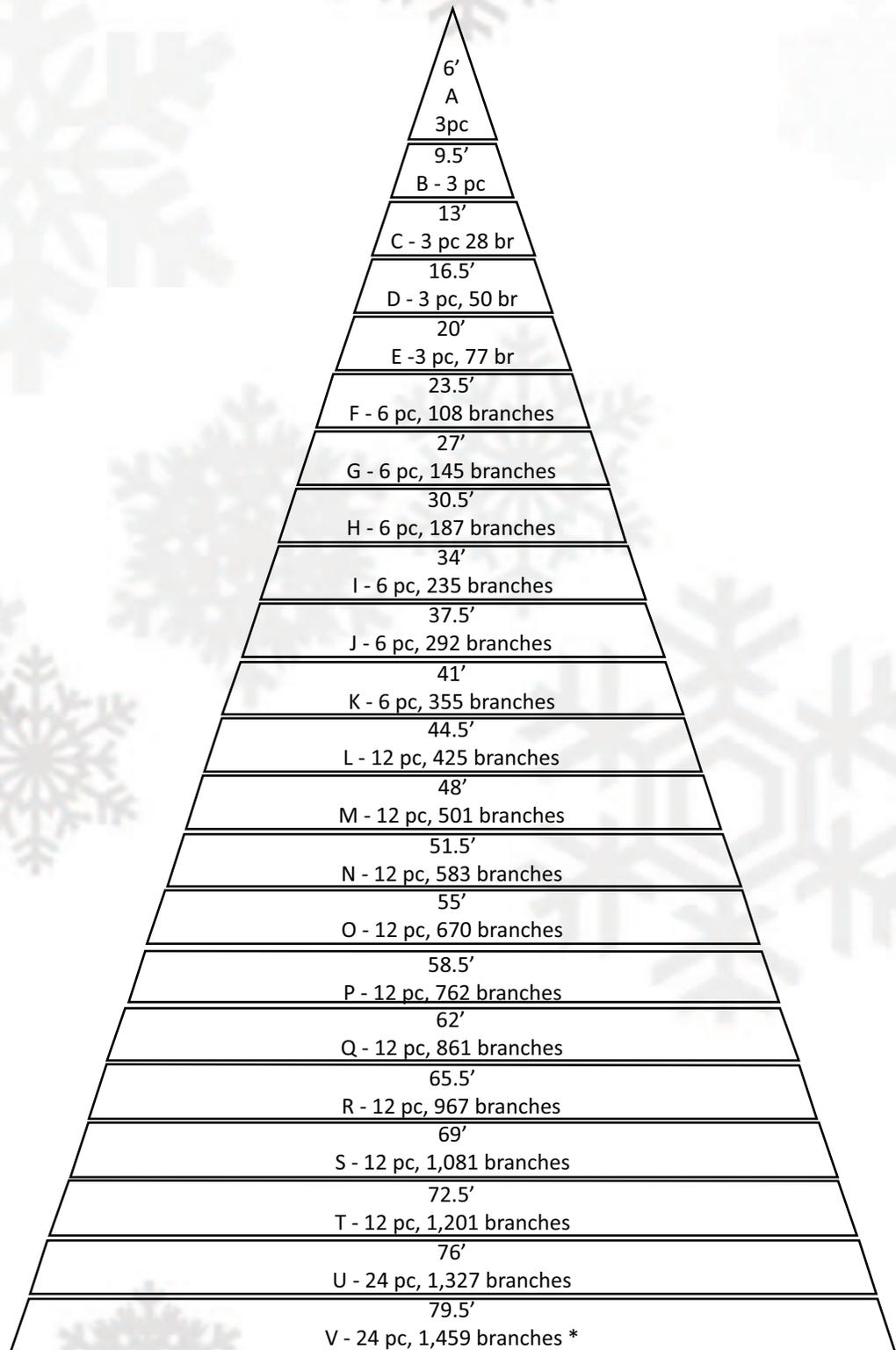
\* Frame pieces needed to build section and running total of branches.
