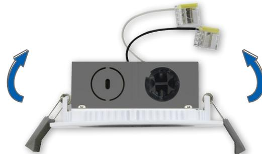
The 4" THINFIT SERIES DOWNLIGHT is designed to be used for both new construction and remodel installations. All wiring takes place inside the integrated J-box which features a pre-installed wire clamp, quick connects and an easily removable lid. After the downlight is wired, simply replace the lid and push the spring action clips into the ceiling cutout. Save time and materials with this easy to install downlight.
