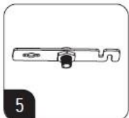
Junction Box Crossbar
