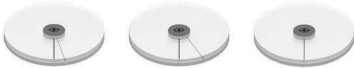
Narrower angle between orientation lines results in more deflection
