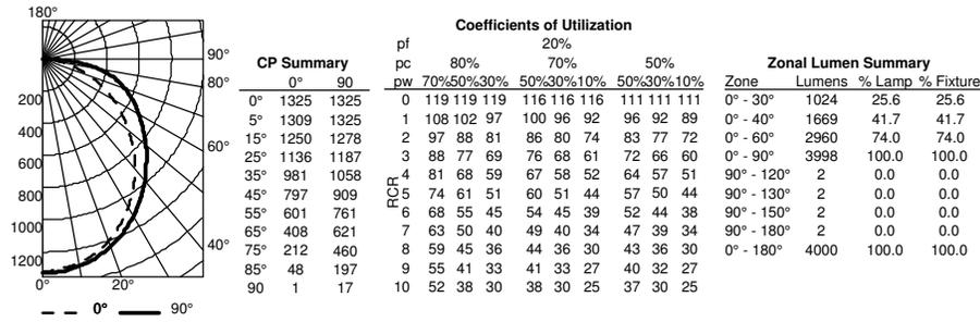
**2BLT4 48L ADP LP835**, 4960 delivered lumens, test no. ISF 36900P117, tested in accordance to IESNA LM-79
