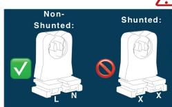
CAUTION: Single-ended input CANNOT be used with shunted lampholders
