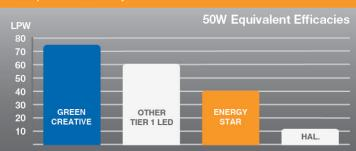
At 75 LPW, this lamp's efficacy is 20% higher than the Tier 1 LED GU10 50W replacement industry average and exceeds ENERGY STAR directional lamp requirements by upwards of 88%. This energy-saving performance makes this lamp a smart retrofit choice for halogen bulbs.
