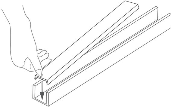
**2.** Press in the subsequent sections of the cover. Be careful not to bend or break the wings of the cover.
