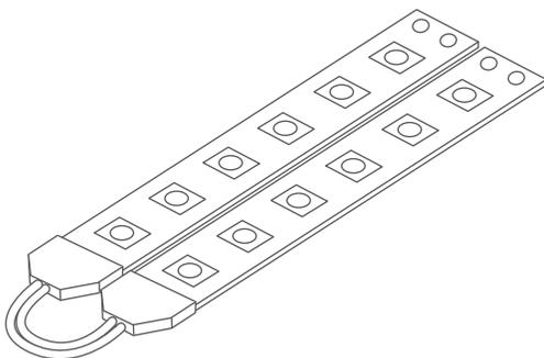
**OPTIONALLY:** The power cords can be led out from one pole of a given strip. This method is used to power suspended lighting fixtures.
