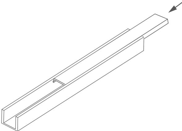
**3.** Insert an end cap into the edge of the extrusion. Individual extrusions have a shape that allows easy installation of dedicated end caps.
