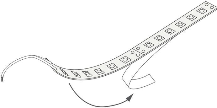
**2.** Attach the tape in the extrusion using the adhesive provided on the LED strip.
