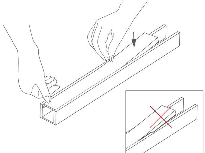
**OPTIONALLY:** Short sections, can also be inserted from the edge of the extrusion.
