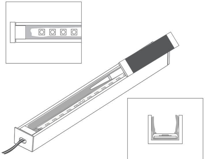
5. Remove the excess silicone with a rectangular tool (e.g. a piece of cardboard), taking care not to damage the tape. The silicone layer must be even and must not obscure the LEDs.
