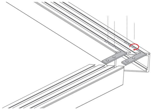
**3.** Slide the other half of the extrusion onto the connectors and tighten the pressure screws with an Allen wrench.
