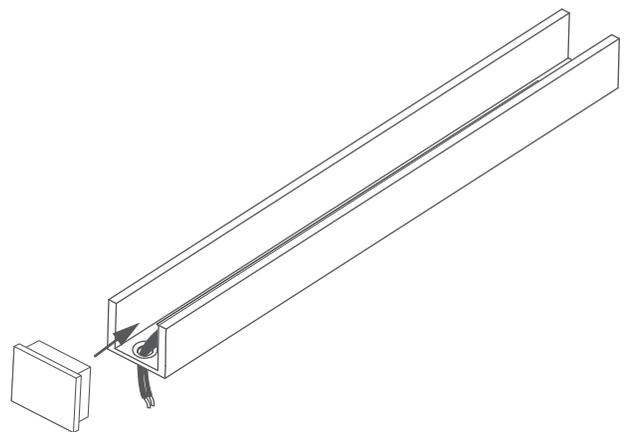
**OPTIONALLY:** The end caps can be attached to the extrusion using glue.
