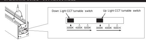
Open the end cap the side with AC wire as the picture shows. Moving the Dip to choose the CCT or you want as the label shows.
