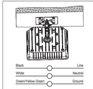
**3:** Attach the Canopy light with bracket by putting the ring on clips again. Connect the Black wire for Line, White for Neutral, Yellow Green for Ground.
