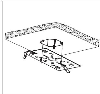
**2:** Fix the bracket on J-box, and put the wire through the central hole for wiring.
