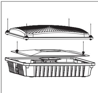
**1:** Remove the lens and metal plate by unscrewing the screws.
