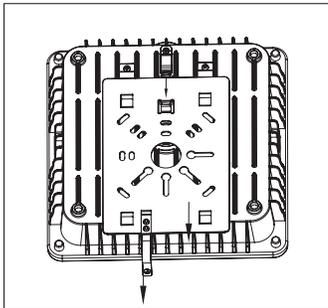
**1:** Loosen the screw on side of the light, removing the bracket from Canopy light by pulling it out slightly, just leaving the ring on bracket.
