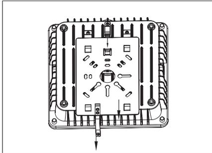
**1:** Loosen the screw on side of the light, removing the bracket from Canopy light by pulling it slightly out, just leaving the ring on bracket. ( See the Step 1 above)
