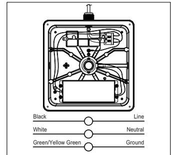
**4:** Disconnect the wires came from 3/4" hole and connect the wires came from 1/2" conduit with power supply. (White for Neutral, Black for Line, Yellow Green/ Green for Ground)
