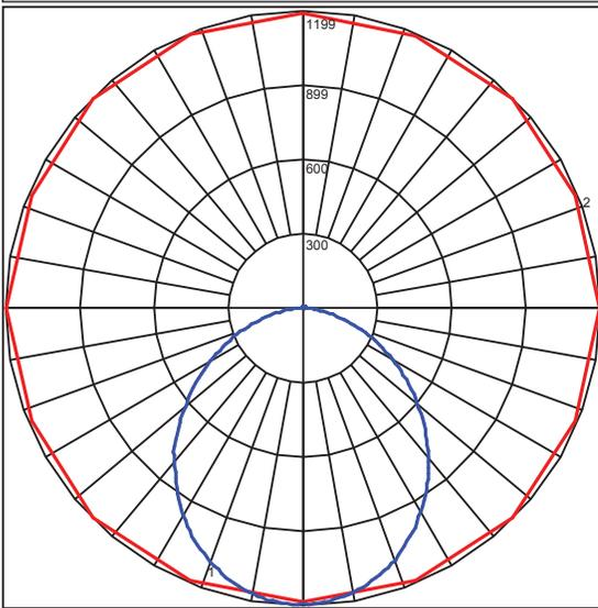
Maximum Candela = 1199.2 Located At Horizontal Angle = 180, Vertical Angle = 2
