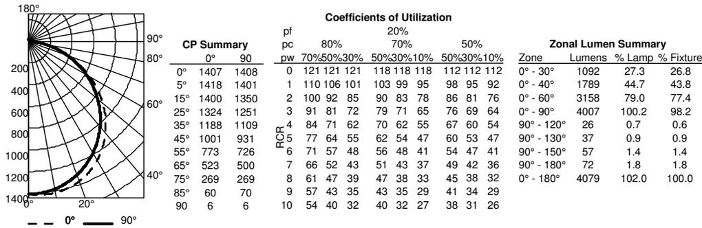
EPANL 22 34L 40K, 3479 delivered lumens, tested in accordance to IESNA LM-79.
