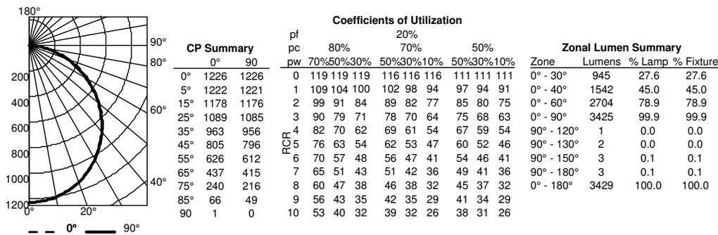
EPANL 24 40L 40K, 4351 delivered lumens, tested in accordance to IESNA LM-79.
