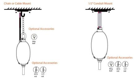
NOTE: PLT-12684 & PLT-12949 use M10-rod. PLT-12685 uses 1/2"-rod. All three use the ring bolt.
